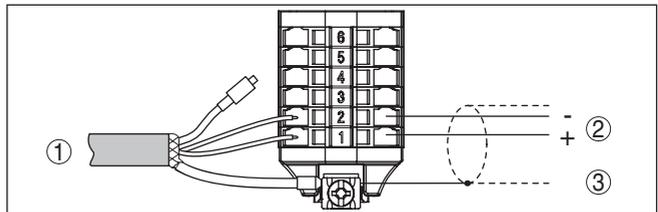
Fig. 11: Schéma de raccordement VEGAWELL 52 4 ... 20 mA, 4 ... 20 mA/ HART
